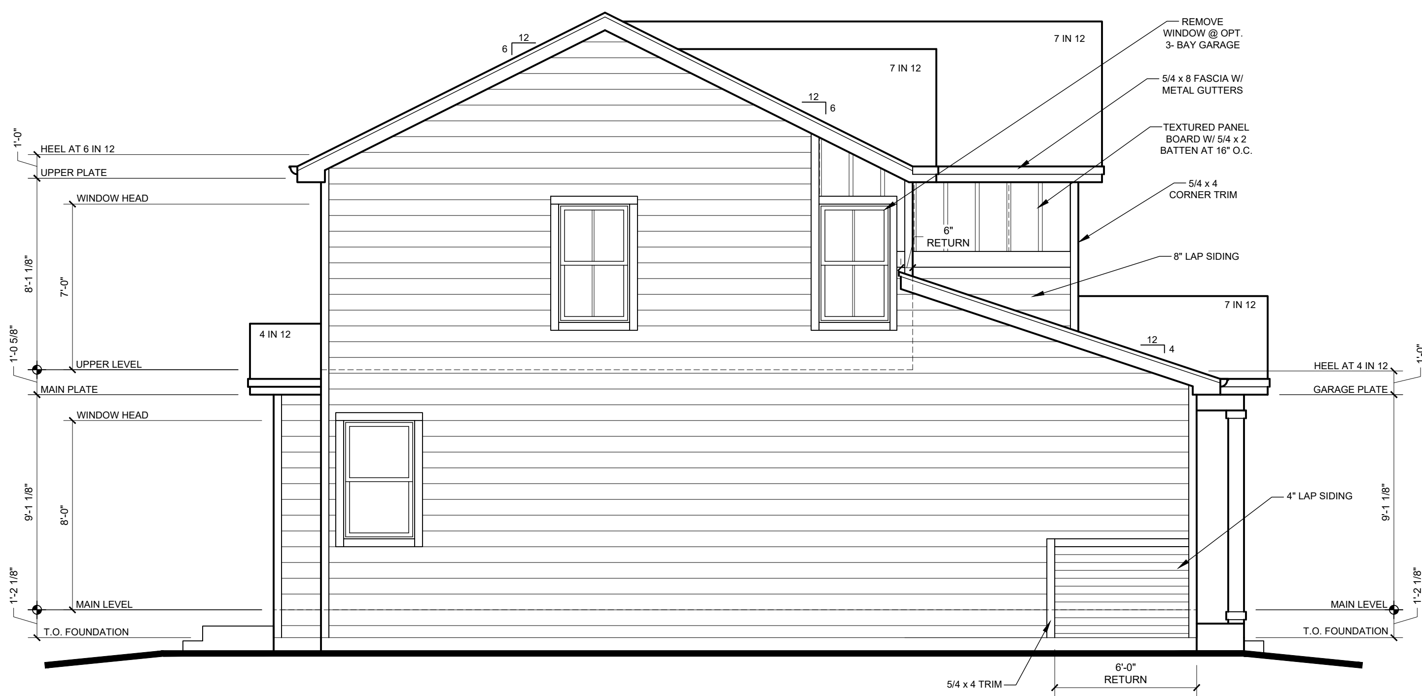
2 GARAGE SIDE ELEVATION - 'A'
