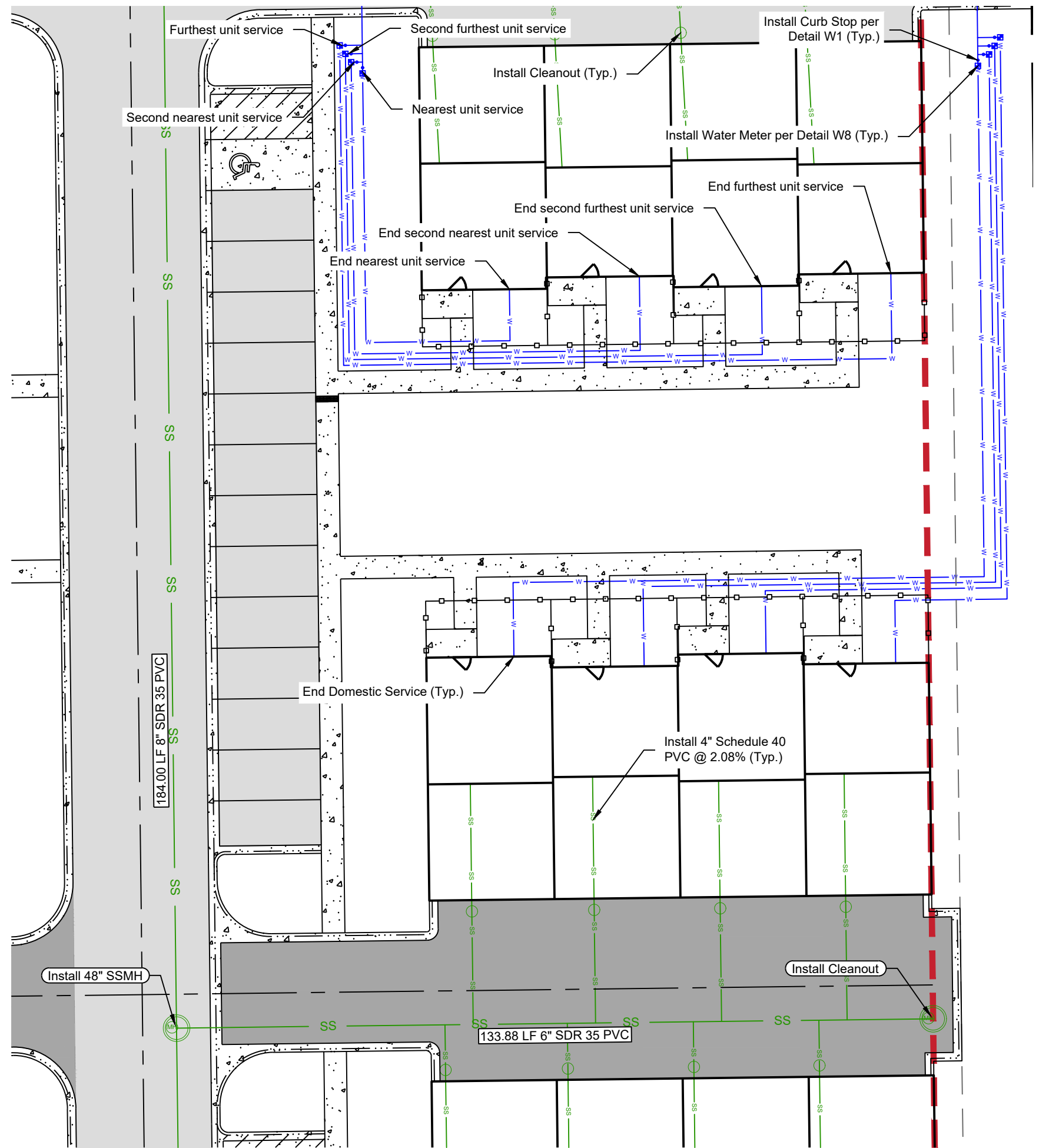
Typical 4-Plex Utility Service Layout Scale: 1" = 20'
