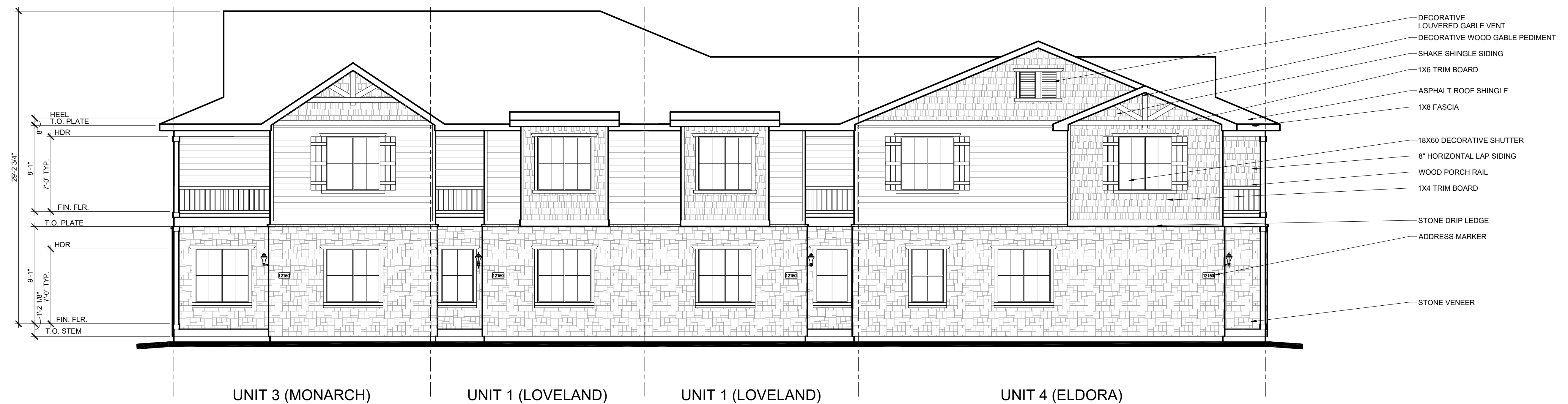
FRONT ELEVATION ELEVATION B 3/16" = 1'-0"
