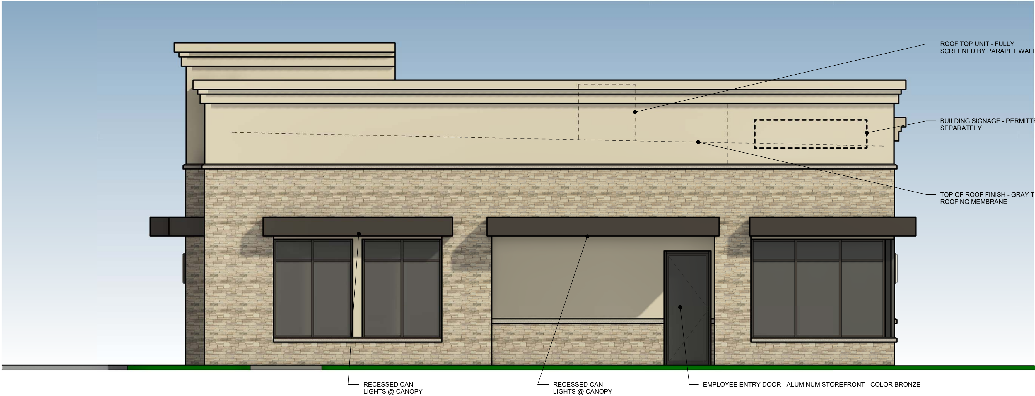
EXTERIOR ELEVATION - SOUTH FACING 1/4" = 1'-0"
