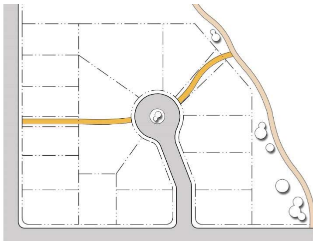
3-4 Walkways and Bicycle Routes. Where streets will not connect or where larger blocks are platted, connections for pedestrians or bikes may be required through blocks or at the ends of disconnected streets. (3.01.B.3).
