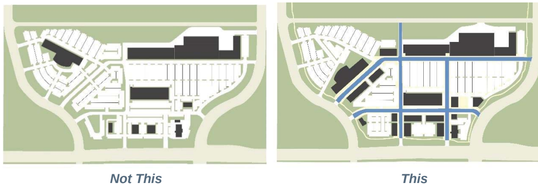
Figure 3-2 Through Access Drives. Through access drives shall be used to mimic public street networks and streetscapes for oversized parcels and large scale development (3.01.B.2.d).
